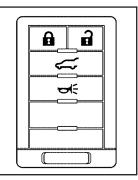
**(Lock):** Press this symbol on the RKE transmitter to lock the doors. This also arms the theft-deterrent system. See *Theft-Deterrent System on page 112* for additional information.
